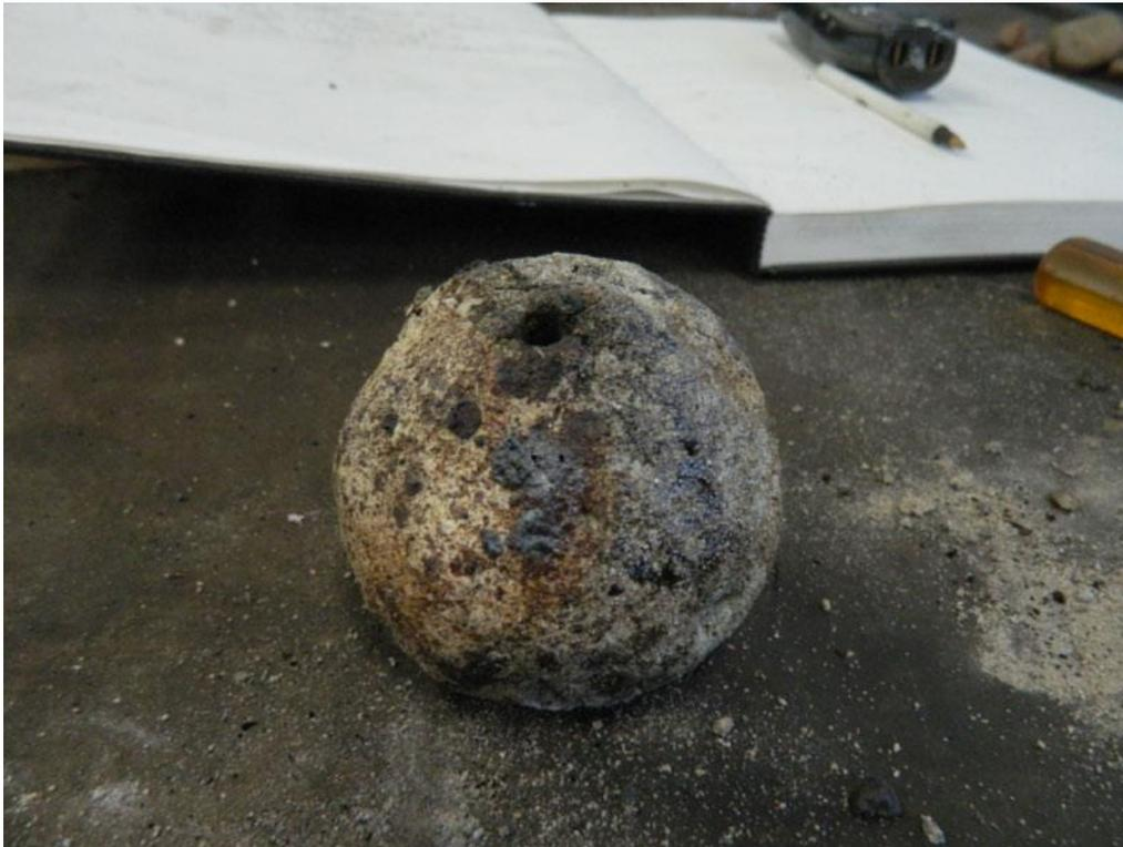
The photo below shows the dumpling cracked open, revealing the bead of iron. In this case, the 25 g of ore yielded a 13g bead of iron. It seems my good ores give 12 to 15 grams of iron.
